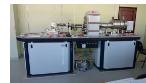
High intense X-ray source with Gallium liquid anode.
